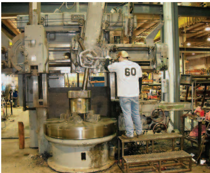
King Vertical Boring Mill with Newall DP7 2-Axes DRO. Part name: Rotary Table Master Bushing. Machinist: Chip Boothe.
